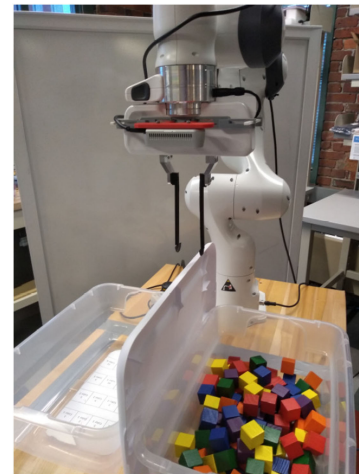
Fig. 4. Franka Emika Panda setup with adapted fingertips.
